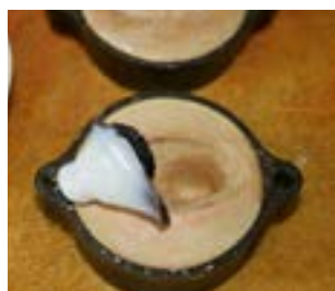
Figure 10 Fit surface showing mechanical retention
