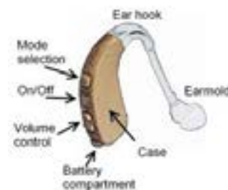
Figure 2 Hearing aid component parts
