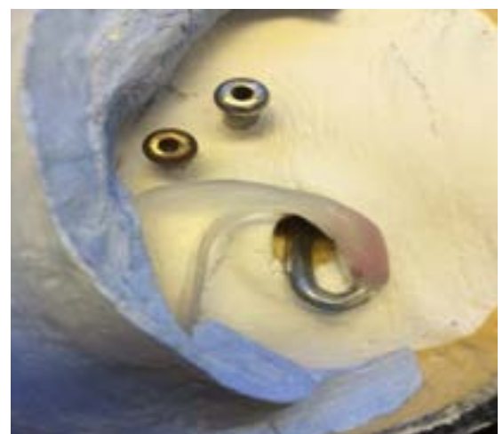
Figure 3 Prototype hearing aid secured into mould
