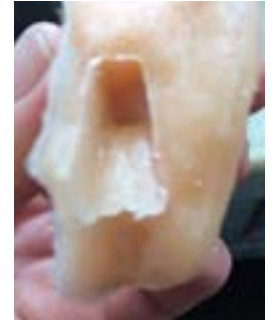
Figure 7 Void on prototype removal
